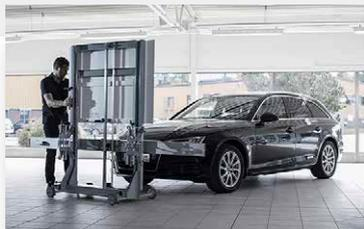
The calibration rig is mounted on a trolley making it easy to move and adjust.
