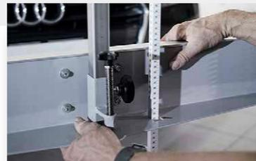
Lift or lower the panel for a parallel alignment by means of a lever.
