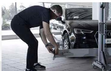
Adjust the cross member (up to 1 m) to correspond with the radar calibration.
