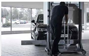
Adjust the upper reference panel to the height in accordance with manufacturer specifications (1.85 m for transporter). Exact positioning is made easier with the help of spring relief.
